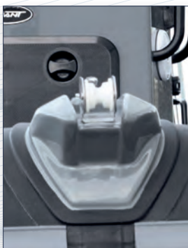
Fibreglass bow platform with bow roller
